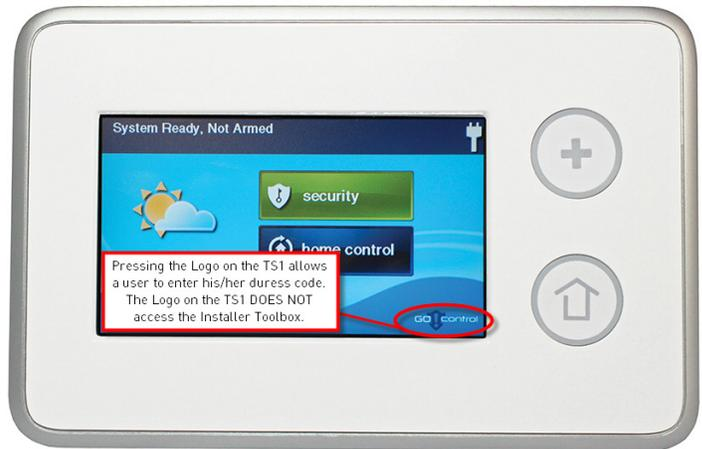
If a user presses the logo on the bottom corner of the TS1 **Home Screen**, the user can enter the duress code only. Installers must remember that the Installer Toolbox can only be accessed from the Control Panel. The TS1 cannot access the Installer Toolbox.
