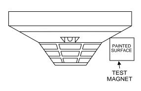
B. Test Module (System Sensor Model No. MOD400 or MOD400R)
