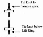
**Type D**: Thread Motor Rope through existing connector or pulley of Lift Ring. When "closed" mark on Rope is in connector, tie triple half-hitch or suitable knot to secure Rope. Or, drill 1/8" hole vertically through Lift Ring. Thread Motor Rope through hole and tie knot. Knot **must** be large enough to prevent Rope from slipping though hole in Lift Ring.
