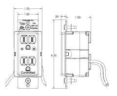
The CA3500 Split-Duplex Receptacle is a Z-Wave™ enabled device which is fully compatible with any Z-Wave enabled network. Z-Wave enabled devices display the Z-Wave logo and guarantee connectivity and interoperability between devices. Each line powered node in a Z-Wave network is designed to act as a repeater forming a mesh network eliminating radio "dead spots" and providing the highest level of reliability.
