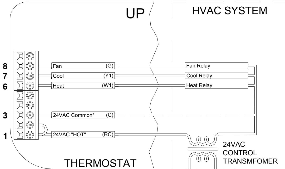
\* Common wire is required in "heat only" or "cool only" applications. Also use a common if heat, cool, or fan relay cannot supply 15mA to power thermostat, without activating.
