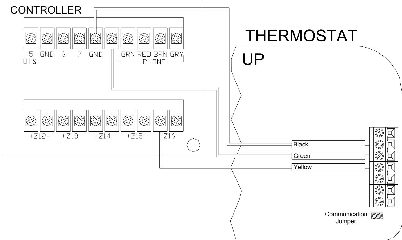
**Figure 9 – Connections to HAI Home Control System**
