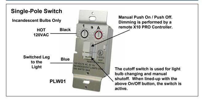
**Description:** The PLW01 Wall Dimmer Switch is designed to control incandescent bulbs (only) with a rating of 40 to 500W. Bulbs rated below 40W may flicker and/or operate erratically. A pushbutton is provided for local On/Off control. A Power Cutoff Switch located directly below the Local On/Off Pushbutton is provided for bulb changing. Both switches should line-up for normal operation.
