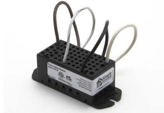
Anywhere Virtual Fixture (Relay) Module Junction box mount or break away ears for tighter fit 6" stranded #14 AWG wire connections, requires hot and neutral Model: UFR-V0
