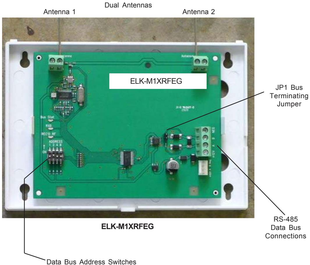
NOTE: Jumper JP1 makes it convenient to terminate the RS-485 Data Bus if this is the last installed device.
