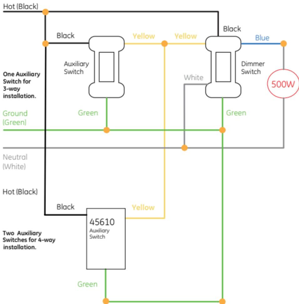
Up to 2 Auxiliary switches may be used to create a 4-way installation
