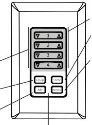
Multi-color LED (Green/Orange/Red) (behind bezel). Visible only when the device is in setup mode
